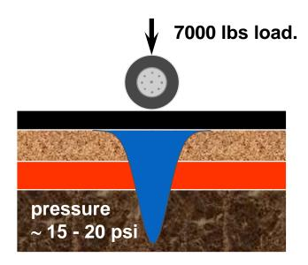
Concrete's rigidity spreads the load over a large area & keeps pressures on the subgrade low (therefore the flooded support system does not impact the load carrying capacity to the same degree as asphalt)
