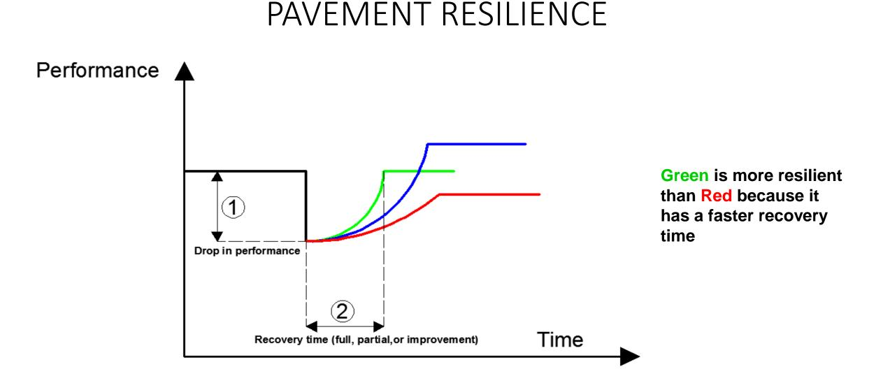
**Pavement Resilience** with respect to an event (eg. Flooding) is characterized by two parameters:
