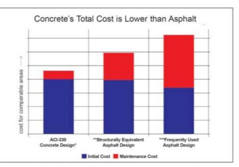
Concrete parking delivers value: Factoring initial placement, maintenance and repair costs, compared to asphalt, concrete costs less over its useful life.
